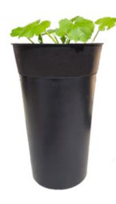
This Adosia SPACE-powered self-watering pot prototype determines when to begin the watering cycle based on the soil (or medium) moisture level. The self-watering pot example uses a BluPonix SPACE subassembly with a single submersible water pump, water level sensor switch and analog soil moisture sensor.
