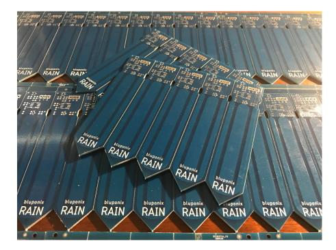
Adosia's RAIN Analog Soil Moisture Sensor for our BluPonix line is based on a modified open design hardware design (thanks DFRobot). Design, schematic, layout, prototype spin and delivery all within 2 weeks from start to finish.
