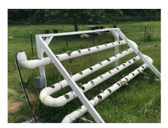
This functional hydroponic snake uses Adosia's BluPonix SPACE v2.2 hobby kit in hydroponic cycle mode. The dual pump channels are used to transport water from the reservoir to the top of the snake. Digital IO #1 is wired to an external solenoid water valve to refill the main reservoir when water level sensor switch #1 is triggered. Digital IO #2 is wired to a separate external solenoid water valve to refill the dogs' water bowl when needed.
